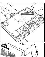
Remove the replacement belt from the storage channel.
